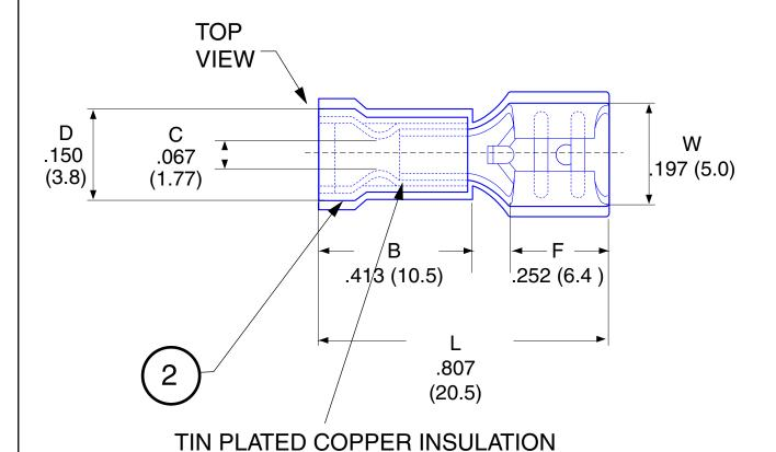
Max Electric Currrent: 22-16 AWG : 10 Amp Max Electric Rating: 75° C / 600 V Max Tolerance ±.05
