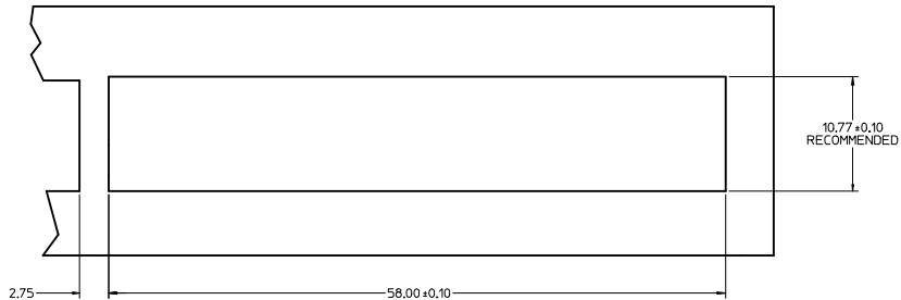
BEZEL AND BOARD POSITION DIMENSIONS FOR SINGLE SIDE MOUNTING
