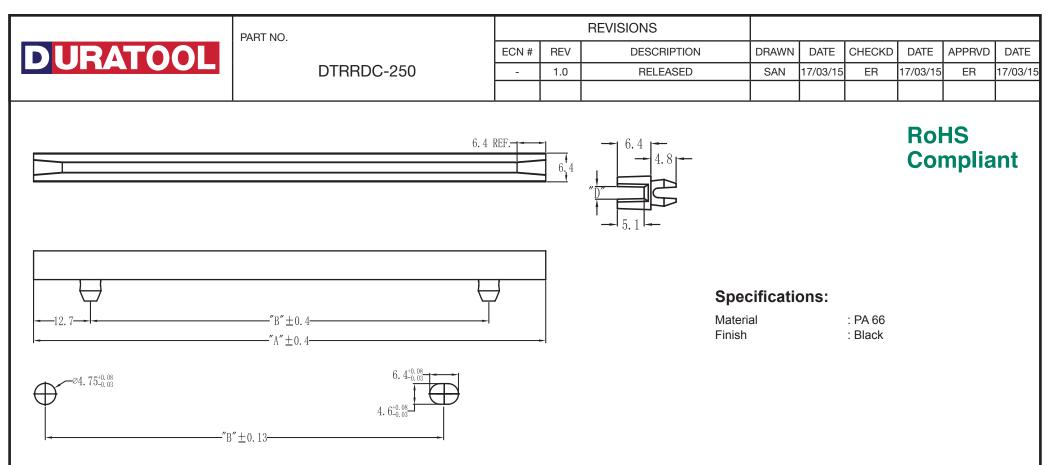
ASSEMBLE HOLE PLATE THICKNESS: (1.2-2.3)
