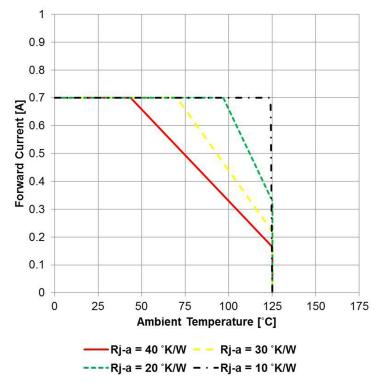
Rja = Thermal Resistance between the junction and ambient
