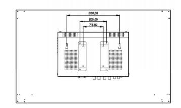
Line Drawing for: Model No. L240SDI All sizes are in mm Drawing not to scale.
