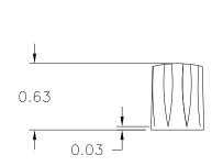
USE #36 DRILL(Ø1065), 6-32 TAP 6-32 X 1/8, CUP POINT, SLOTTED, SET SCREW, I0511 0.50
