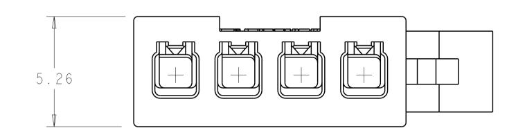
THIS DRAWING IS A DIMENSIONS: mm MATERIAL NYLON, UL 94V - 0 NATURAL
