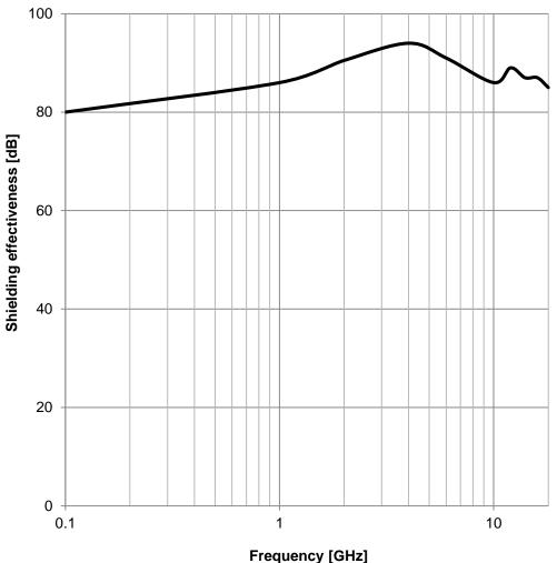
GENERAL TOLERANCE CREATED CHECKED Würth Elektronik eiSos GmbH & Co. KG EMC & Inductive Solutions KaS JoV DIN ISO 2768-1m Max-Eyth-Str. 1 74638 Waldenburg **WE-LT Conductive Shielding** Tel. +49 (0) 79 42 945 - 0 Gasket ORDER CODE www.we-online.com 3021001 eiSos@we-online.com REVISION STATUS DATE (YYYY-MM-DD) BUSINESS UNIT PAGE Square 005.000 Valid 2017-01-16 eiSos 2/3 **WÜRTH ELEKTRONİK**
