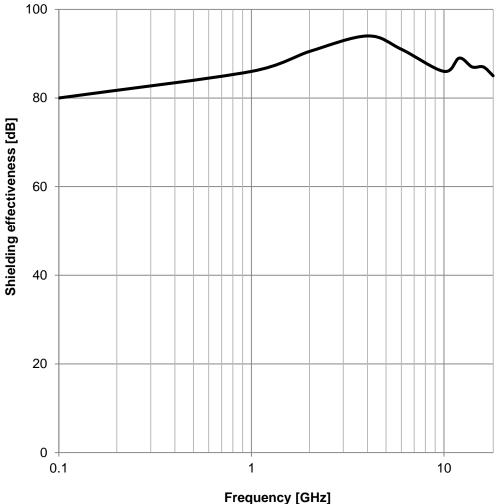
GENERAL TOLERANCE CREATED CHECKED Würth Elektronik eiSos GmbH & Co. KG EMC & Inductive Solutions KaS JoV DIN ISO 2768-1m Max-Eyth-Str. 1 74638 Waldenburg **WE-LT Conductive Shielding** Tel. +49 (0) 79 42 945 - 0 Gasket ORDER CODE www.we-online.com 3021508 eiSos@we-online.com REVISION STATUS DATE (YYYY-MM-DD) BUSINESS UNIT PAGE Square 004.000 Valid 2017-01-16 2/3 eiSos **WÜRTH ELEKTRONİK**
