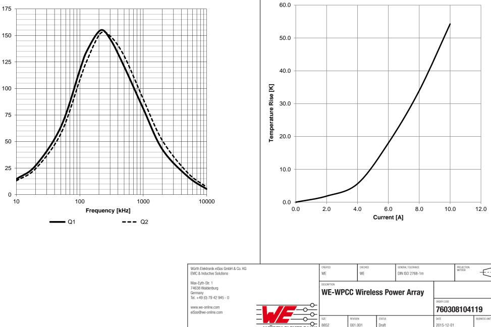
**Typical Temperature Rise vs. Current Characteristics:**
