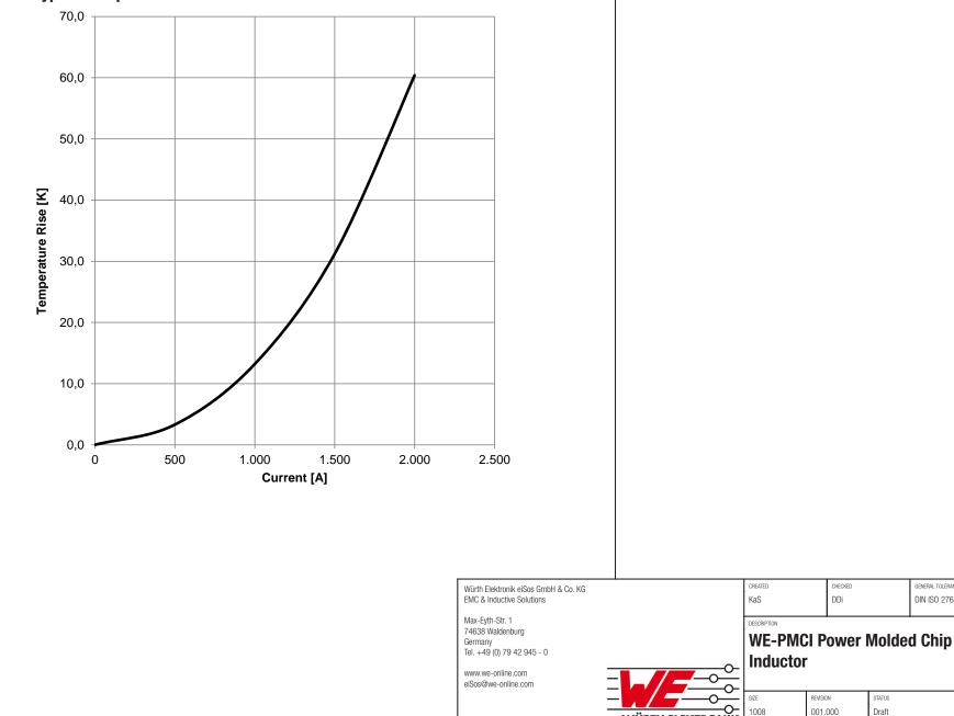
**Typical Temperature Rise vs. Current Characteristics:**
