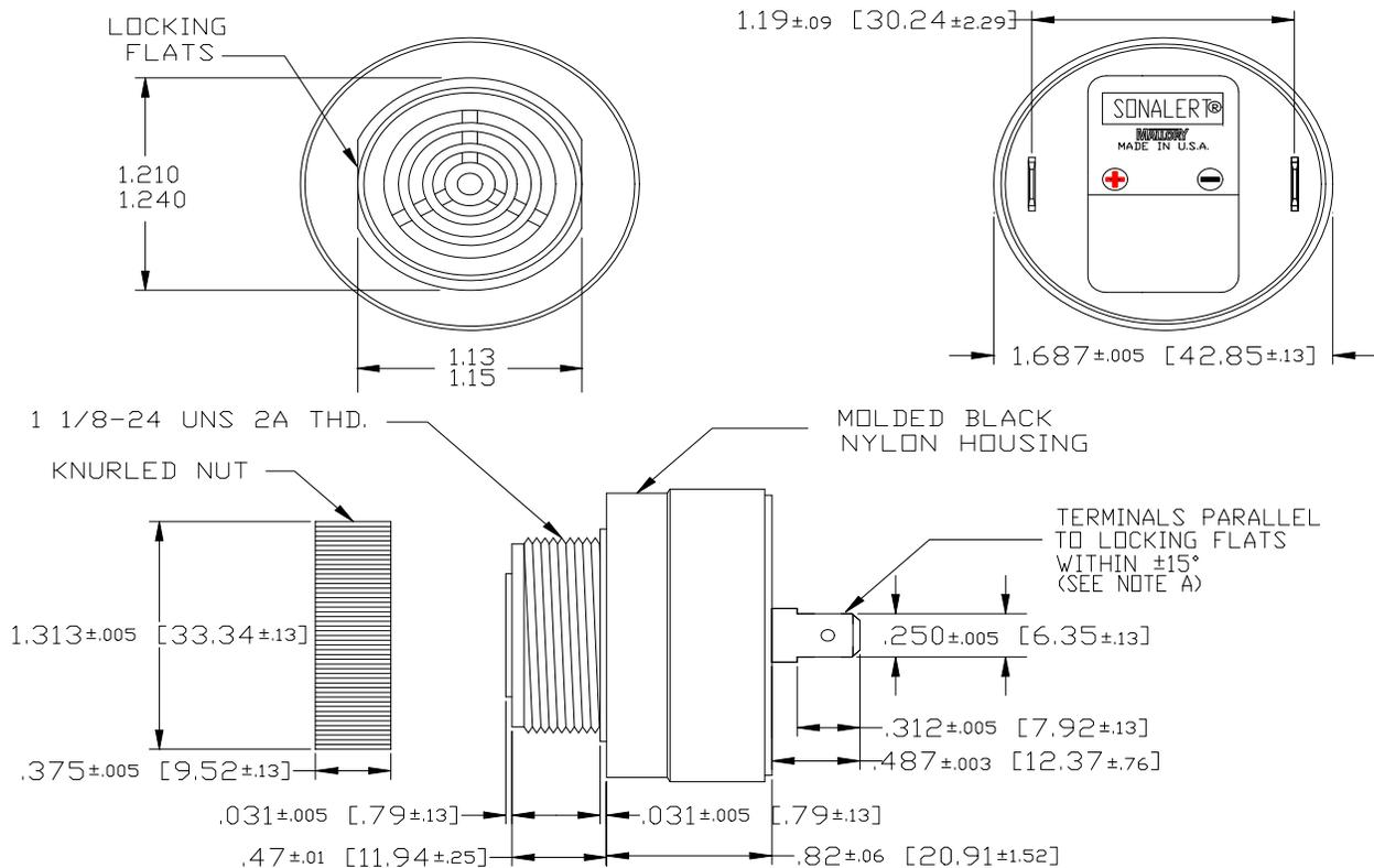
MOUNTING: REMOVE BLACK PLASTIC NUT AND INSERT THREADED FRONT THROUGH 1.25" HOLE PUNCHED IN PANEL, IF ORIENTATION IS NEEDED, NOTE LOCKING FLATS ON DRAWING. SCREW NUT BACK ON. DO NOT OVERTIGHTEN.
