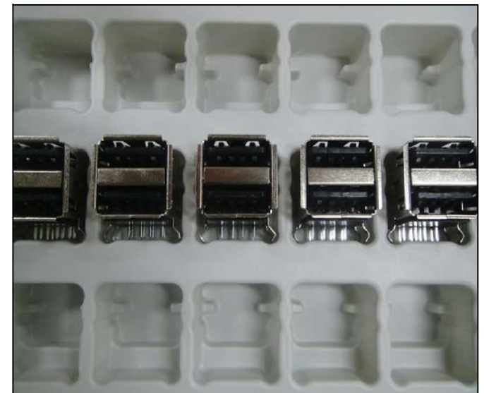
USB's placed into the tray base. 将USB连接器放入吸塑盘内
