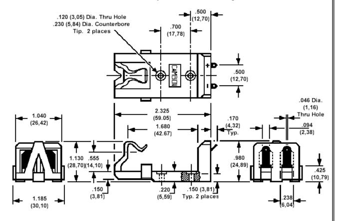
Rec. Mounting Holes - .062 (1,57) Dia., on pitch of 0.500 (12,70) centres, plus bolt down holes per drawing Suited for use on boards up to .125 (3,18) thick
