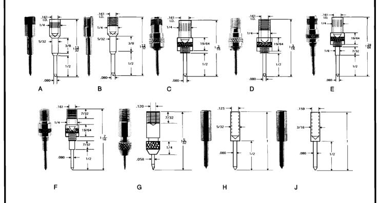
BODY: Brass, Nickel-plated. NEEDLE TIP: Steel, Nickel-plated.
