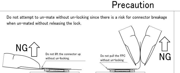
Do not un-mate in the depth direction to avoid contact or housing damage even when the lock is released.
