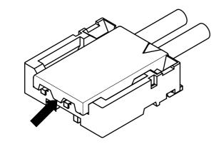
②Lift up to the upper difrection and friction lock is released.
