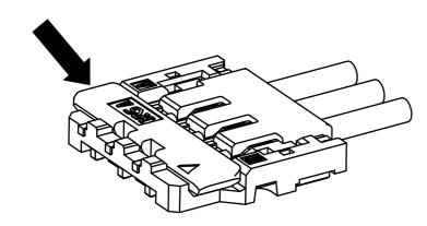
② Lift up to the upper difrection and friction lock is released.
