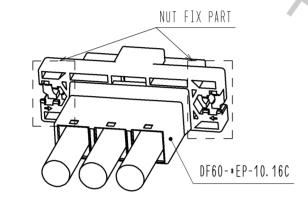
1. SLIDE A NUT (SIZE:M3) TO NUT FIX PART.
