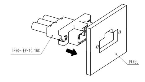
2. TIGHTEN A SCREW (SIZE:M3) TO FIX WITH PANEL. RECOMMENDED TORQUE: LESS THAN 49N·cm
