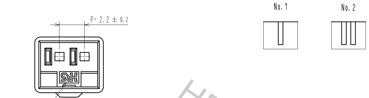
1> FIGURE-1 CONTACT No. MARKING (10:1)
