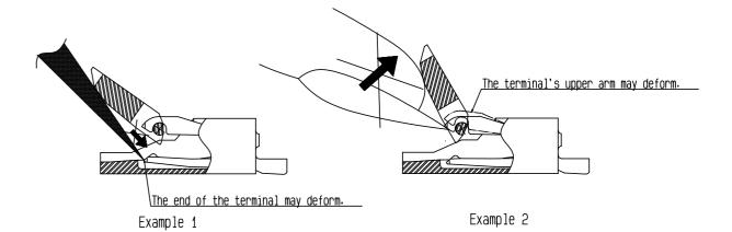
2. When operating the actuator, do not apply a force in the direction of the connector. The actuator may get pushed into the connector, causing damage to the connector.
