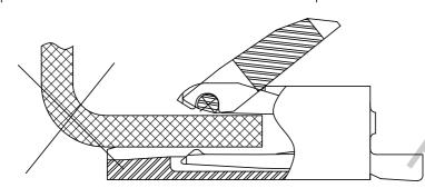
5. When inserting an FPC, do not use the method shown in the photo on the left below where the corner of the FPC is inserted first and then slid sideways. the FPC's corner can deform the terminal's contacts. Always insert the FPC parallel to the board as shown in the photo on the right below.
