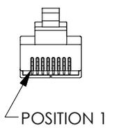
4TP, CAT 5e, 26AWG STRANDED SILVER PLATED COPPER WITH ALUM/POLY FOIL SHIELD AND ROUND TINNED PLATED COPPER BRAID, (85% MIN. COVERAGE).
