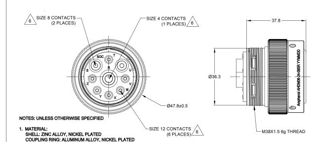
2. MODIFICATIONS: THREADED HOUSING; REDUCED DIA. SEAL
