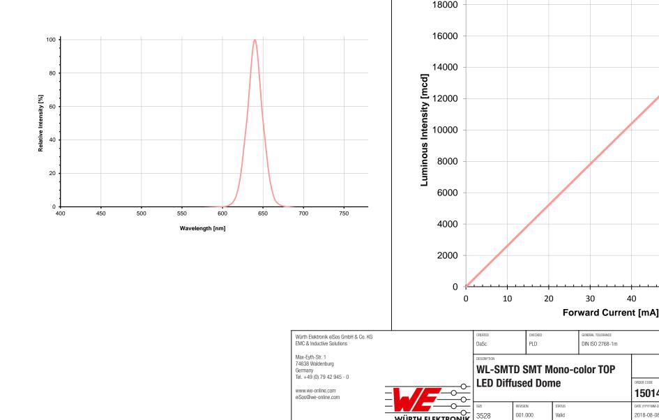
**Luminous Intensity vs. Forward Current:**
