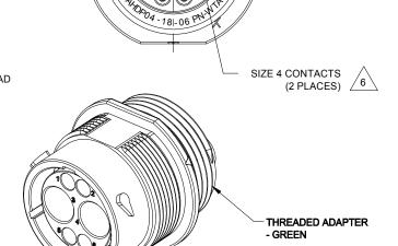
RECEPTACLE, 18-06 POS, PIN CONT., STANDARD DIA. SEAL, AHDF
