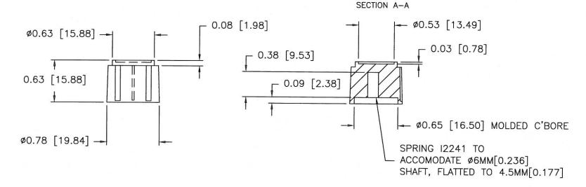
NOTE: ALL MOLDED PARTS MUST BE CHECKED WITH SPECIAL GAUGE. KEYWAY PIN MUST ACCEPT MOLDED HOLE
