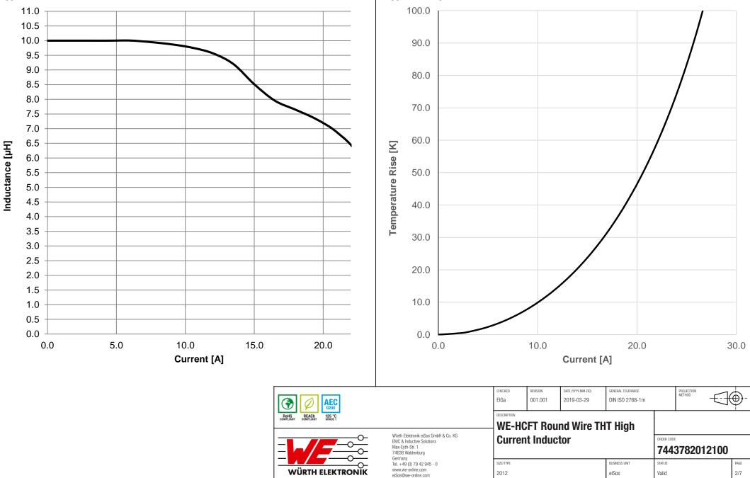
**Typical Temperature Rise vs. Current Characteristics:**
