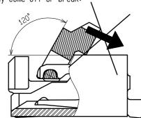
4. Move the actuator at approximately the center. Do not operate the edge of actuator. Otherwise, the actuator may come off or break.
