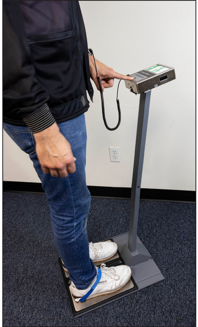
Figure 15. Using the Combo Tester X3 Plus with EMIT 50416 Stand
