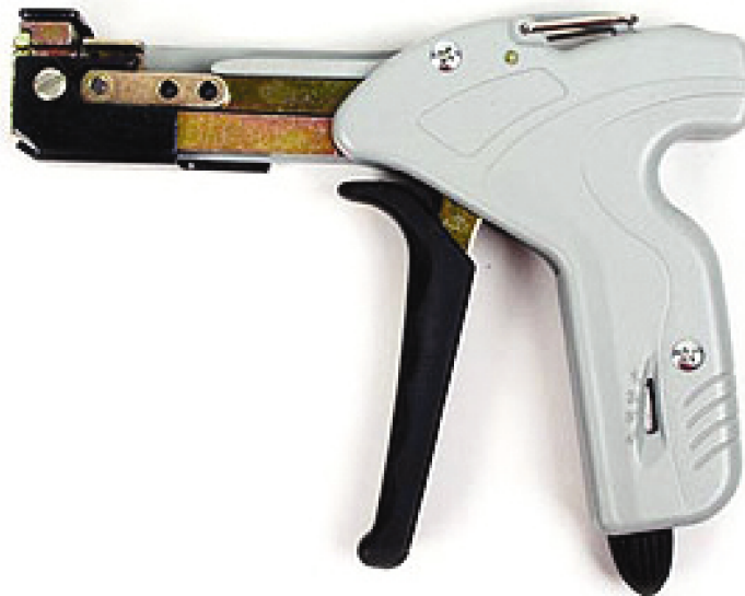
CABLE TIE INSTALLATION TOOL FOR METAL TIES (MT-X SERIES) TIES WIDTH: UP TO 7.9mm [.03 IN] TIE THICKNESS: UP TO 0.3mm [.01IN]
