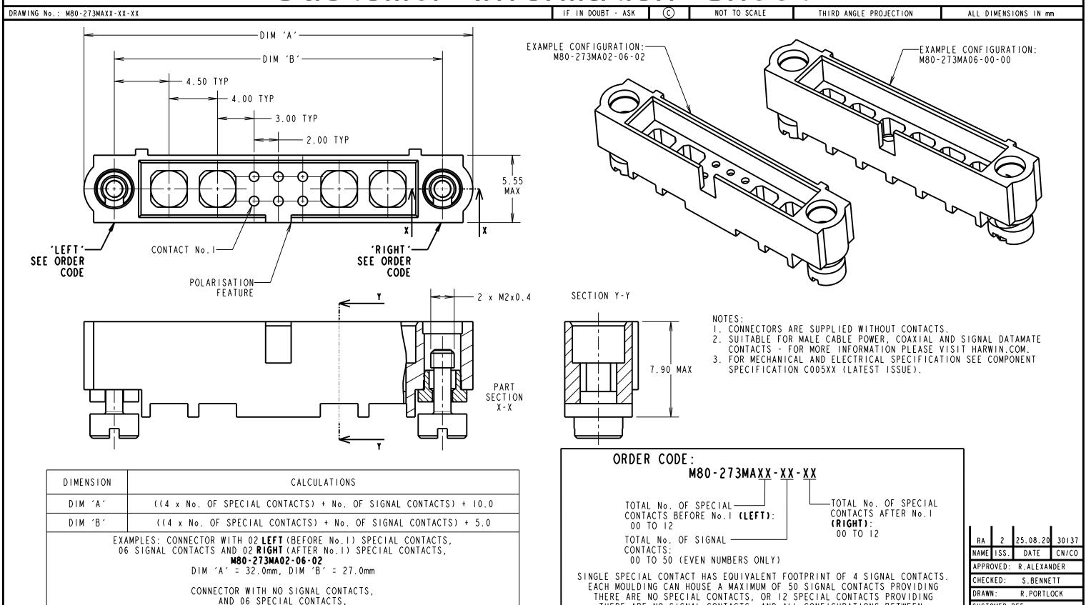
M80-273MA06-00-00 DIM 'A' = 34.0mm, DIM 'B' = 29.0mm
