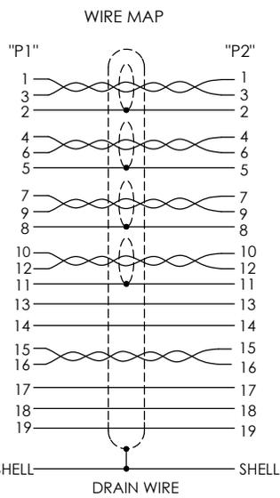
HYBRID TYPE CABLE WITH 50/125 OM3 FIBER AND COPPER CONDUCTORS. ALUM/POLY FOIL SHIELD AND DRAIN WIRE JACKET: PVC, BLACK (O.D.: .177 [4.5])
