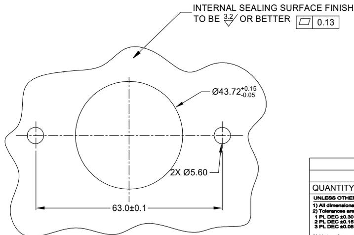
INTERNAL SEALING SURFACE FINISH
