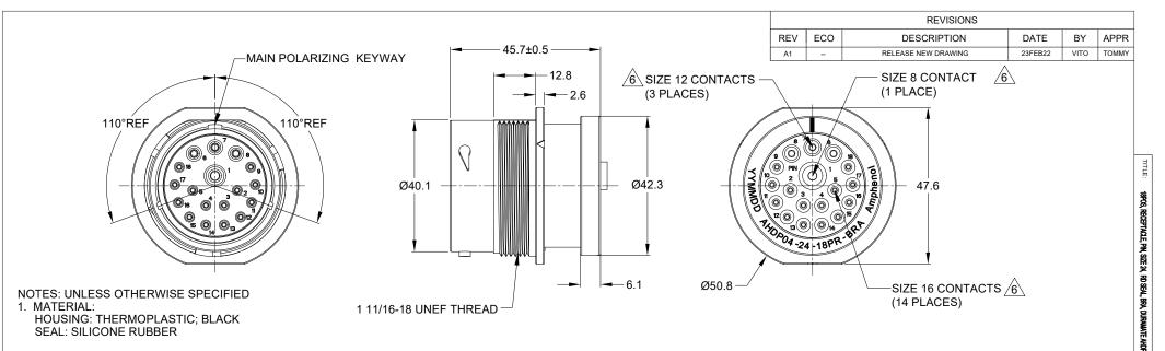
2. MODIFICATIONS: BACKSHELL RING ADAPTER (BRA); REDUCED DIA. WIRE SEAL.
