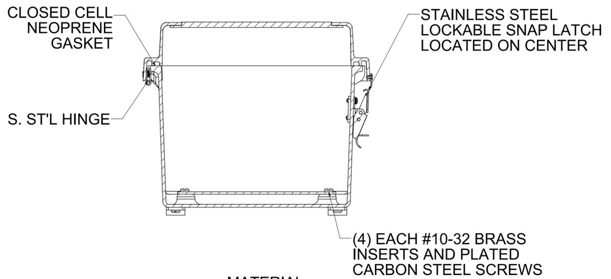
(4) EACH #10-32 BRASS INSERTS AND PLATED CARBON STEEL SCREWS
