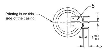
Note: No welding onto the groove
