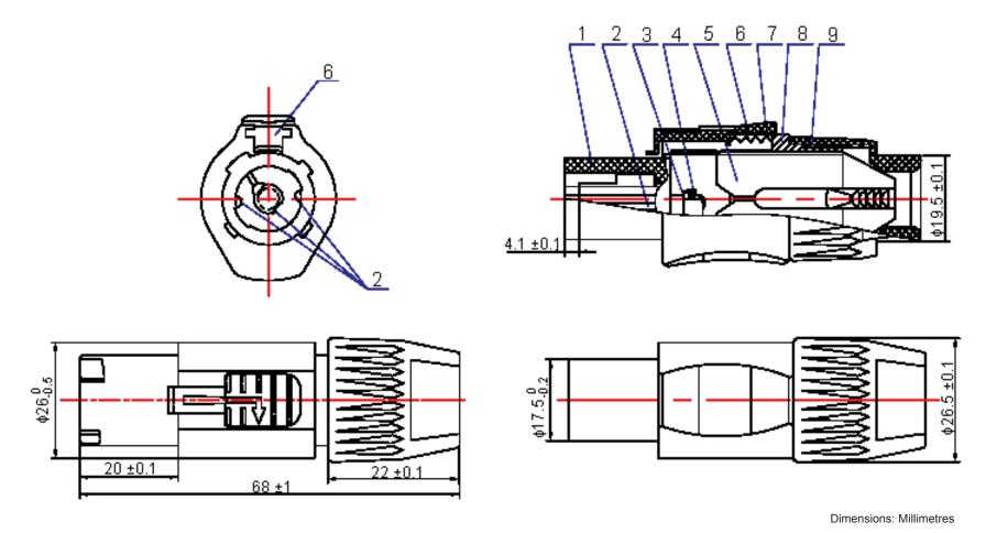
The pin plating silver, thickness 0.5µm (SOLDER+SCREW).
