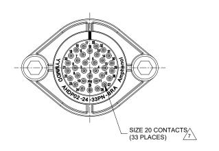
33 POS, RECEPTACLE, PIN, PANELMATE AHDP SIZE 24,NORMAL SEAL, BRA
