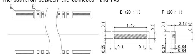
Connector lead on PAD layout ☐ PAD layout
