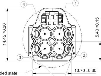
Envelope Ø16.3mm in final assembled state
