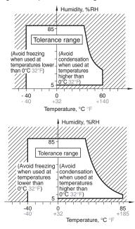
\* –40 to +85°C –40 to +185°F (When 45% to 80%V of coil holding voltage)
