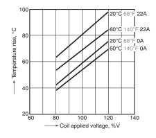
2. Ambient temperature characteristics and coil applied voltage
