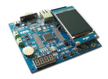
this board, which enables engineers to evaluate the full features of the STM32F107VC processor and accelerate to design and develop their own projects based on this processor.
