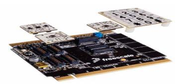
S08QE96 microcontroller on board, the TWR-SENSOR-PAK module can be used stand-alone or as part of a complete Tower System.
