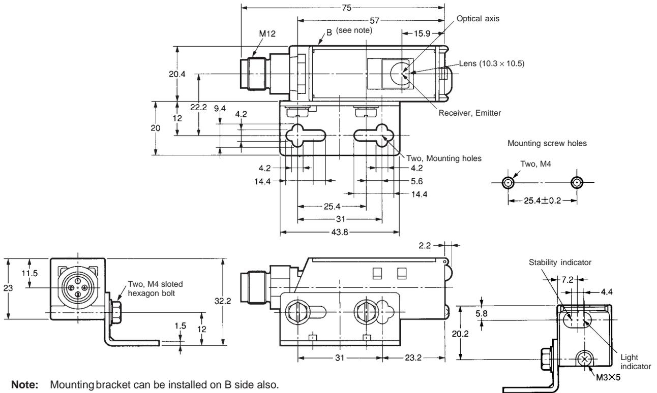
**Note:** Mounting bracket can be installed on B side also.
