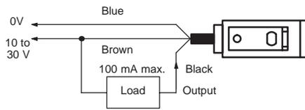
**Note:** If the load is a relay, insert a surge absorbing diode between the coils of the relay.
