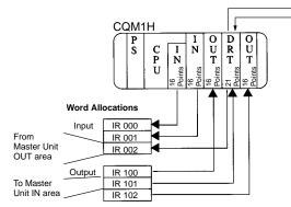
PS: Power supply Unit CPU: CPU Unit IN: Input Unit OUT: Output Unit DRT: I/O Link Unit
