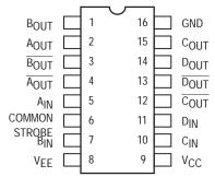
Pin assignment is for Dual–in–Line Package.
