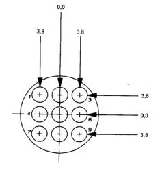
9 Positions Free-Hanging Connector accepts Type III + Contacts Water Protected IP 65
