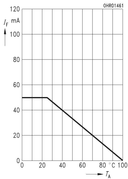
Figure 4. Maximum Permissible Forward Current, I_F = f(T_A) , R_{\theta JA} = 450\text{ K/W}
