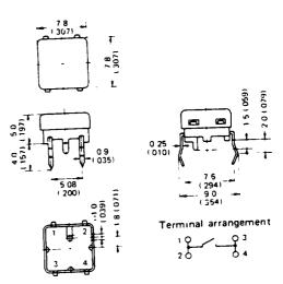
Freedom in PC board mounting is expanded due to microsized and low-profile configuration (ranging from 6.9 mm square × 3.2 mm height to 12.8 mm square × 6 mm height).
