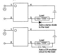
2) Even if spike voltages generated at the load are limited with a clamp diode if the circuit wires are long, spike voltages will occur by inductance. Keep wires as short as possible to minimize inductance.
